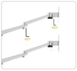
After positioning a proper angle, tighten the frame with a wrench to prevent it from dropping down.
