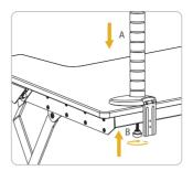
Place the Column (A) on top of the desktop and align to the base screw, then tighten the bolt (B) from the bottom to secure the main column.
