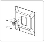
Place the VESA Bracket in position on back of monitor with lip toward top of monitor and attach using 4 screws provided. Use washers if needed.
