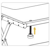
2 Insert the bolt from the bottom of the desktop through any of the 3 buttonhole openings.
