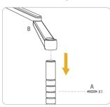
4 Place the rubber ring (A) into the ring groove at your desired height, and then the double section arm (B) is sheathed into the upright column.
