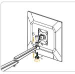
8 Place the Plastic ring(A) into monitor arm hole pattern. Aligh ring to hole pattern. Slide VESA Bracket(B) into arm, fully tighten Clamp Screw(C). Align ring to hole pattern.
