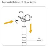
Place the rubber ring (A) into the ring groove at your desired height. Install the dual arm (B) in the post, adjust to the appropriate position, and then use the screw (C) to tighten it.
