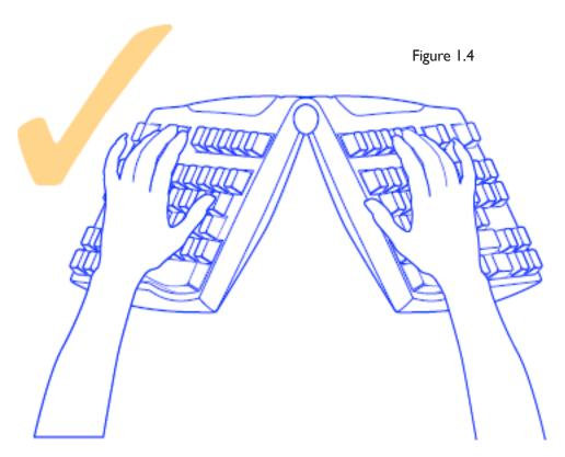
**Important:** Adjusting your keyboard for lateral inclination and pronation relief changes the height of the keyboard. Therefore, it may be necessary to also adjust your seat and desk heights so that the elbows are at 90° and your forearms are horizontal.
