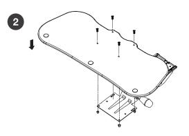
Second, line up the screw holes on the keyboard tray **platform** with the holes on the keyboard mechanism. Line up and insert the 4 M5x15 screws into the indicated holes on top of the keyboard tray platform and line up and place the 4 M5 acorn nuts to the underside of the mechanism. Once in this position, screw in and tighten the M5x15 screws into the M5 acorn nuts.
