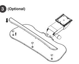
Remove the 3 caps on the end of the keyboard tray and place in a safe location. Attach the wrist rest until you feel all 3 placements have been magnetically secured.
