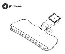
The keyboard tray and wrist rest are securely in place and ready for use.
