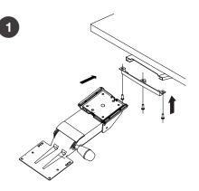
*First*, slide the keyboard tray **mechanism** onto the tracks on the underside of the EasyLift Desk.
